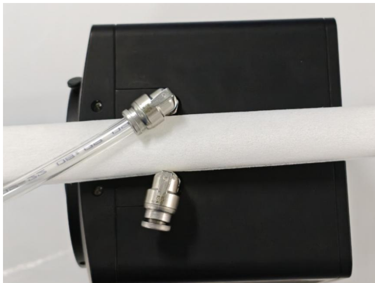
Figure 4-4 Removing water-cooled pipes
