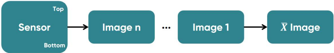
Figure 3-11 Schematic Diagram of Low Noise Mode in Sensitivity Mode
