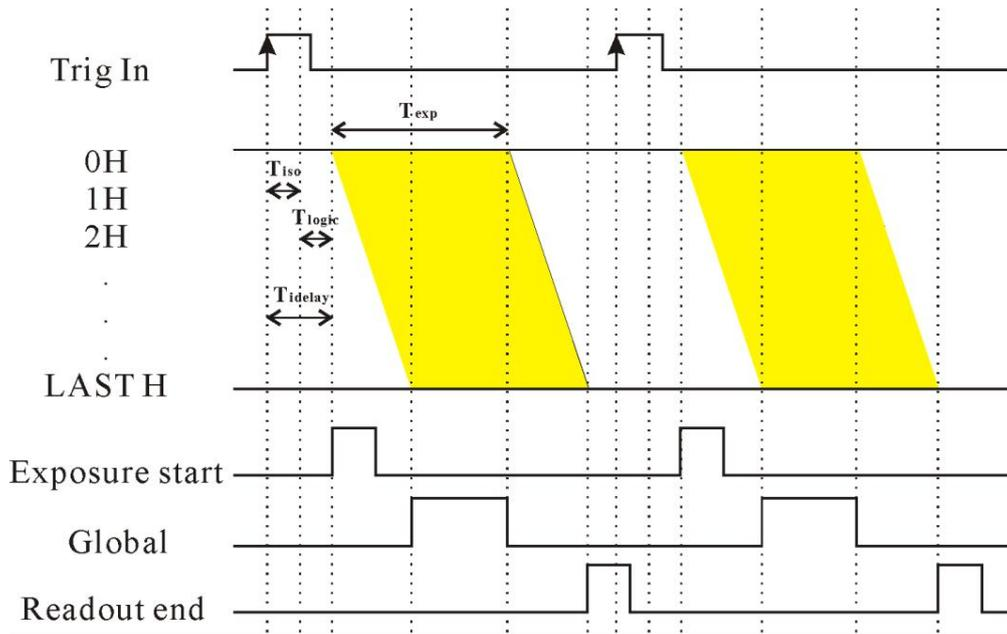
Figure 2-4 The Timing Diagram of Trigger Input&Output
