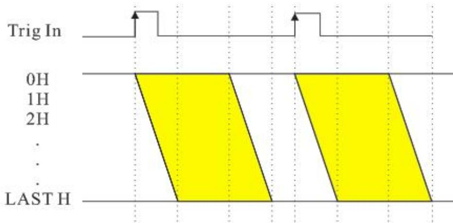
Figure 3-3 Standard Mode (Exposure: Timed / Edge:Rising )
