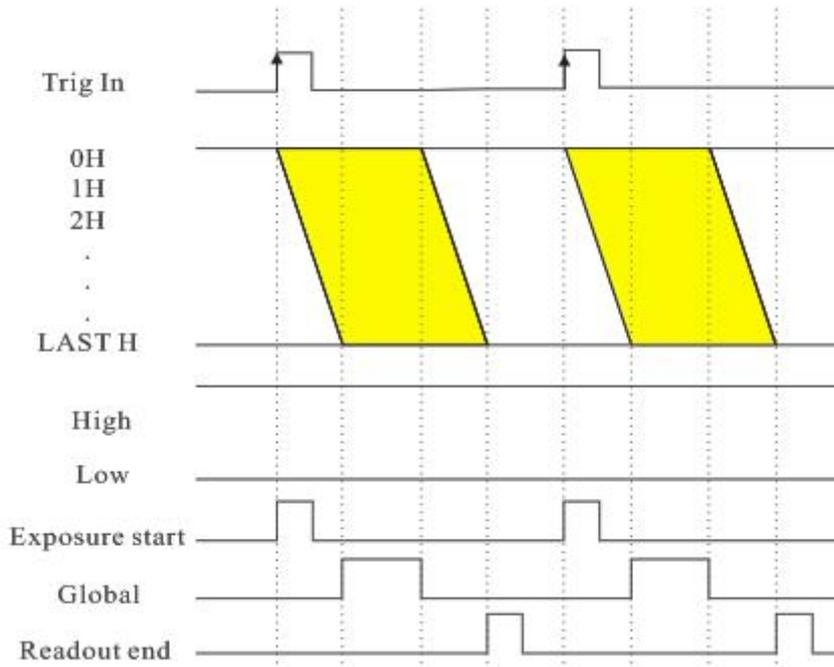
Figure 4-2 Diagram of Output Signal
