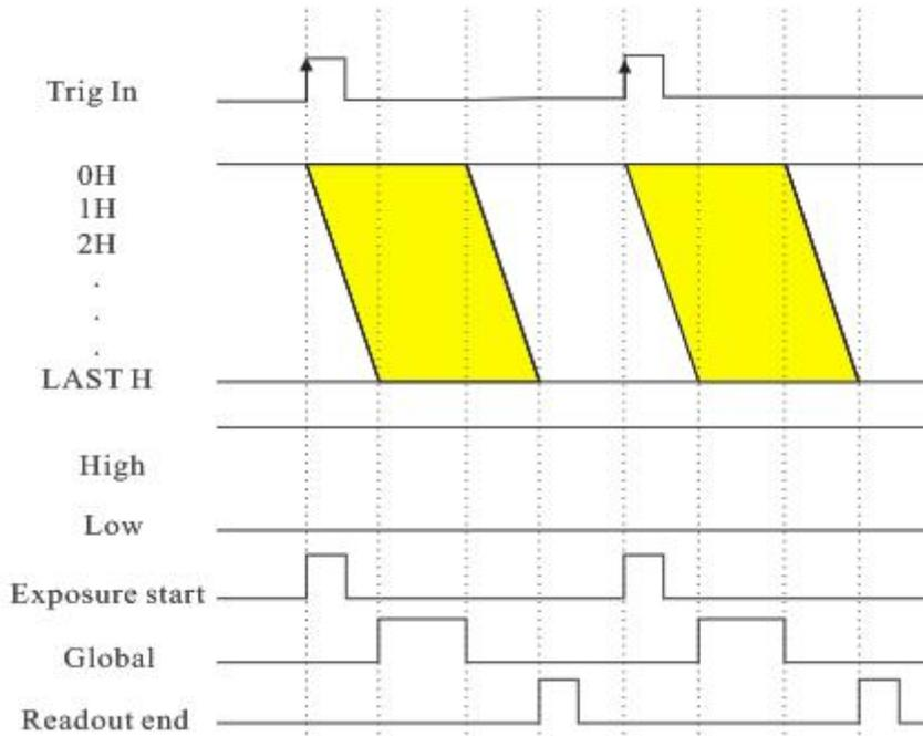
Figure 4-2 Diagram of Output Signal
