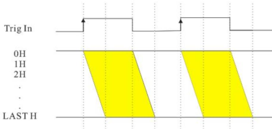
Figure 3-2 Standard Mode (Exposure: Width / Edge:Rising)
