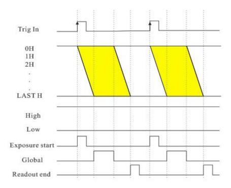
Figure 4-2 Diagram of Output Signal
