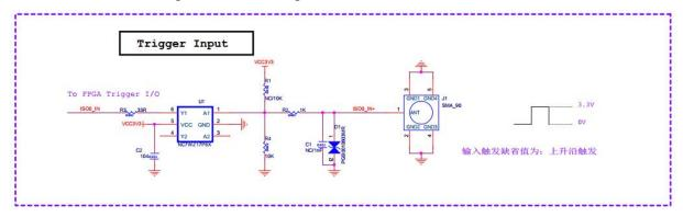
Figure 2-1 Trigger Input Circuit
