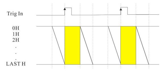
Figure 3-8 Global Mode (Exposure: Time / Edge:Rising)
