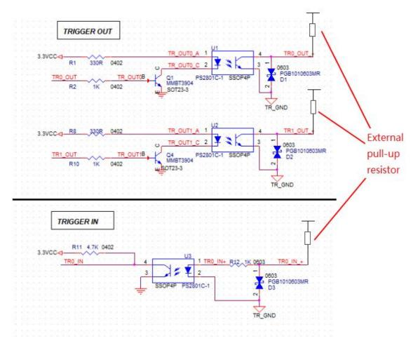
Figure 2-3 FL-20BW/Dhyana 401D Trigger Input&Output Circuit
