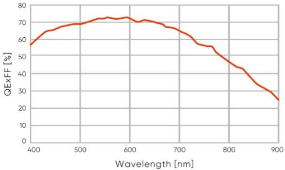
Figure 2-1 Quantum efficiency curve of Dhyana 401D
