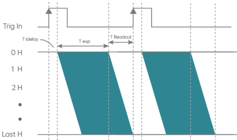
Figure 3-22 Standard (Non-Overlap) Trigger timing
