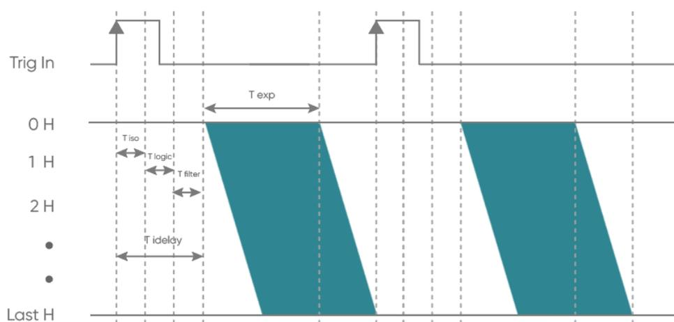
Figure 3-20 Trigger Delay Diagram
