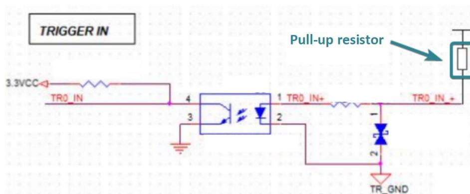
Figure 3-18 Hardware trigger input circuit
