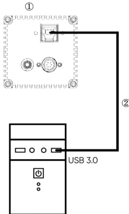
Figure 4-1 Dhyana 401D camera connection diagram
