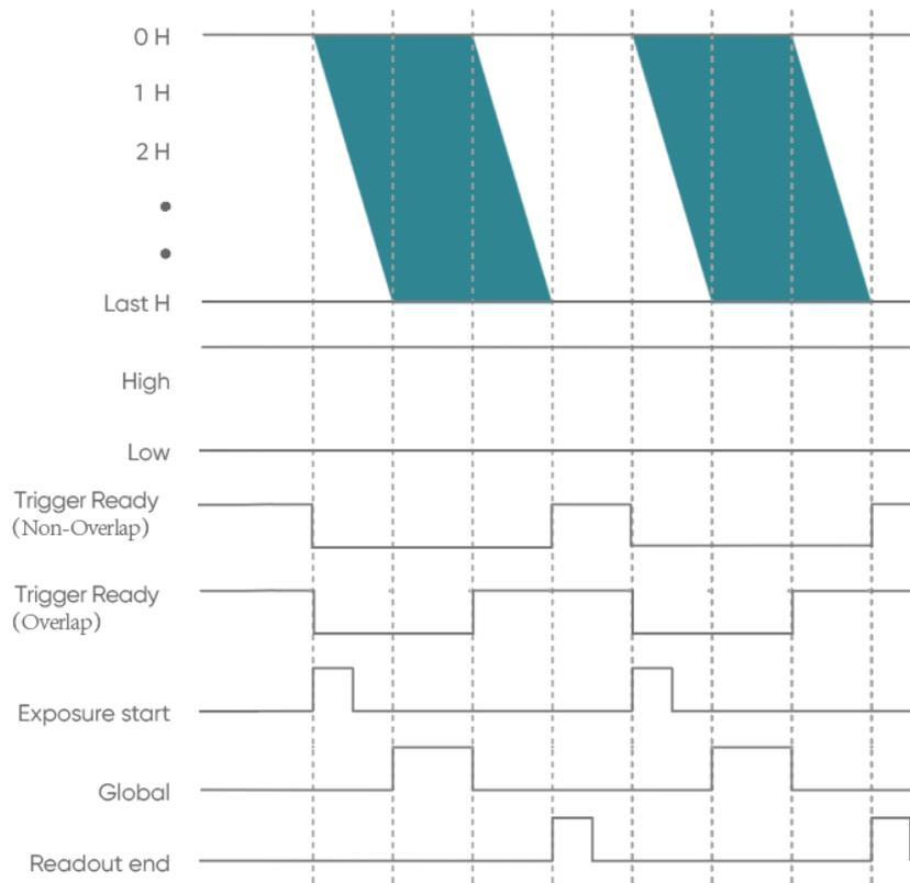
Figure 3-27 Trigger output timing diagram
