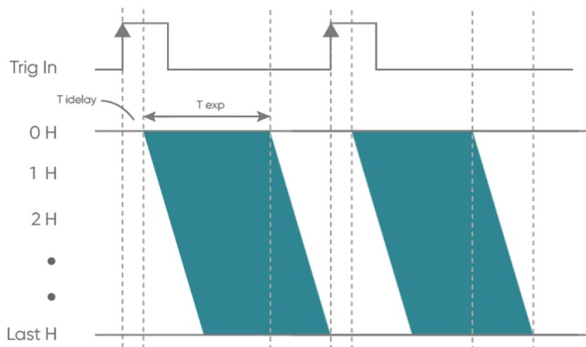
Figure 3-24 Edge Trigger timing diagram
