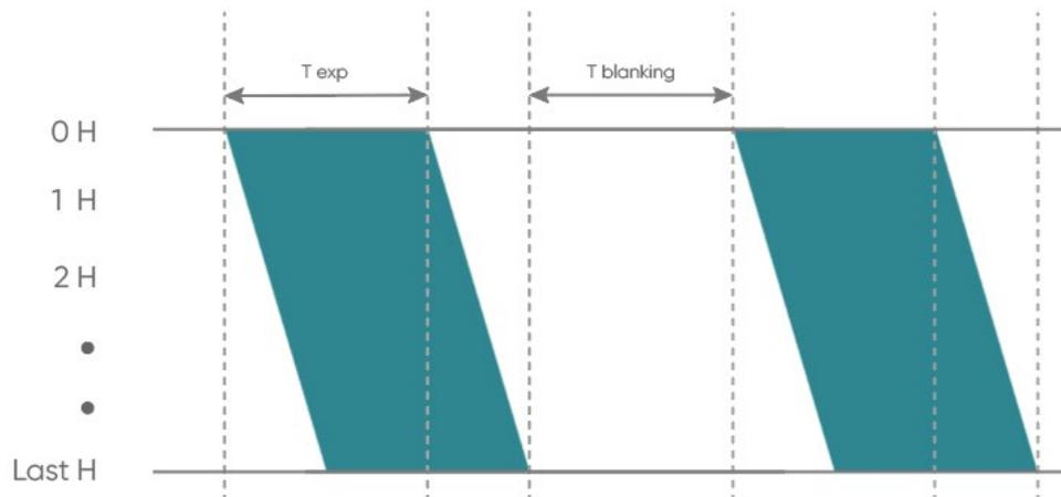
Figure 3-12 Frame rate adjustment timing diagram
