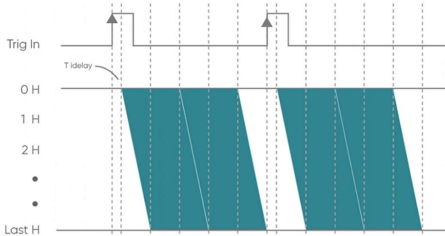
Figure 3-25 Single-trigger multi-frame acquisition timing diagram
