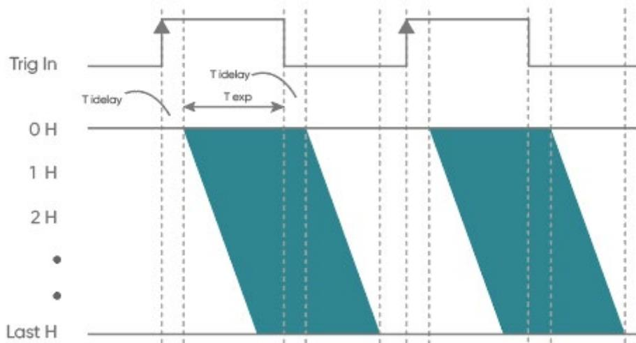
Figure 3-23 Non-Overlap Level Trigger timing diagram
