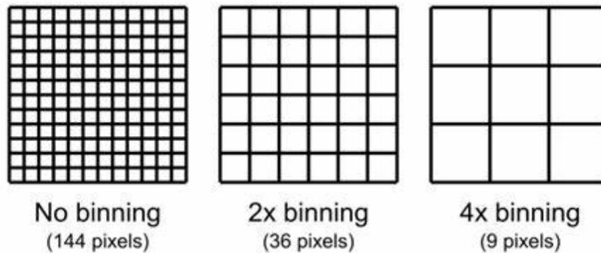
Figure 3-8 Schematic diagram of Binning
