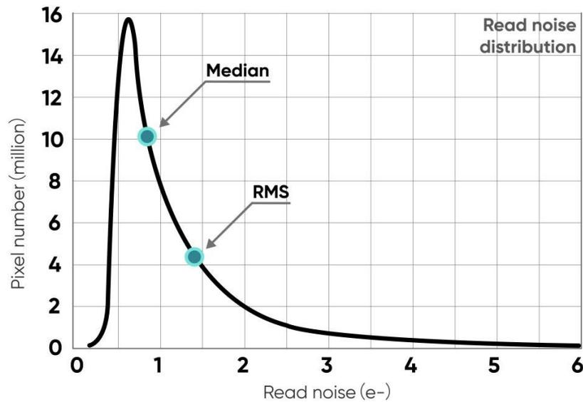
Figure 3-4 Readout noise distribution of an typical sCMOS camera
