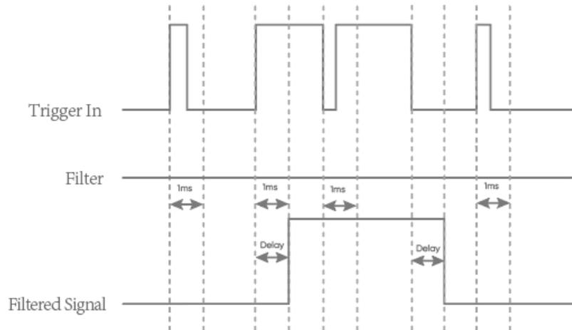
Figure 3-19 Trigger Filter function schematic
