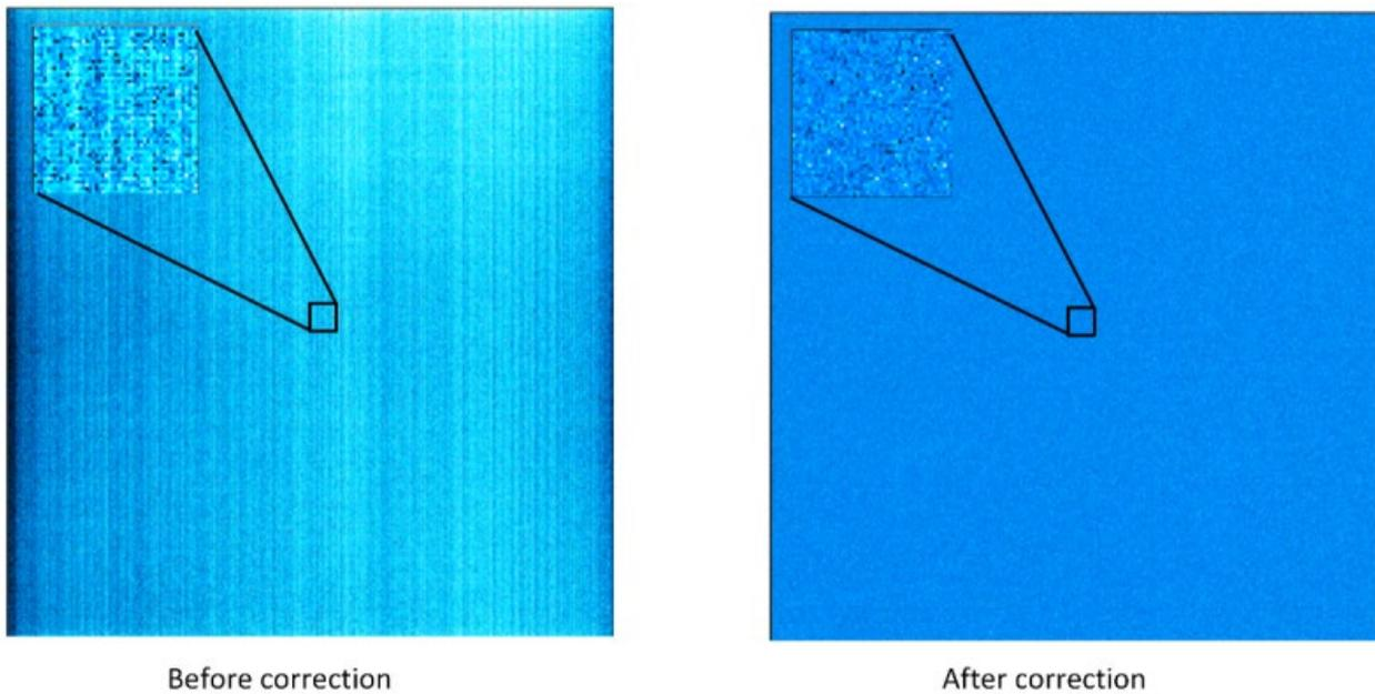
Figure 3-5 DSNU correction comparison before(left) and after(right)
