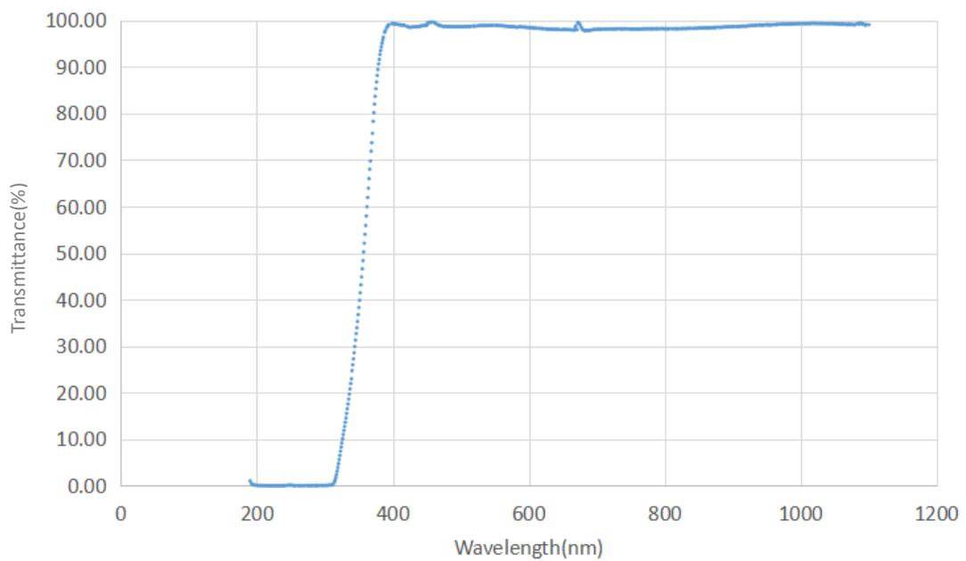
Figure 2-2 Transmission curve of a standard glass window
