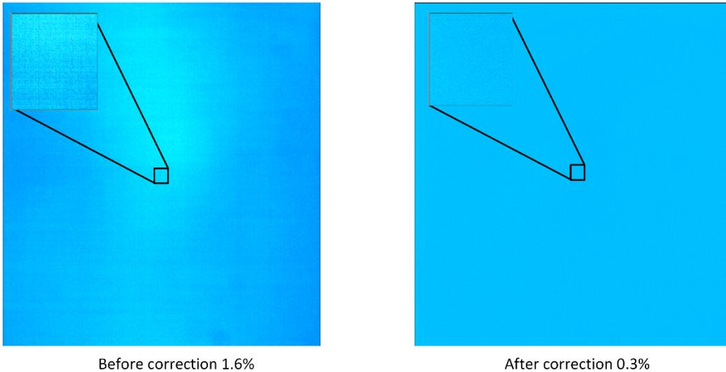
Figure 3-6 PRNU correction comparison before(left) and after(right)
