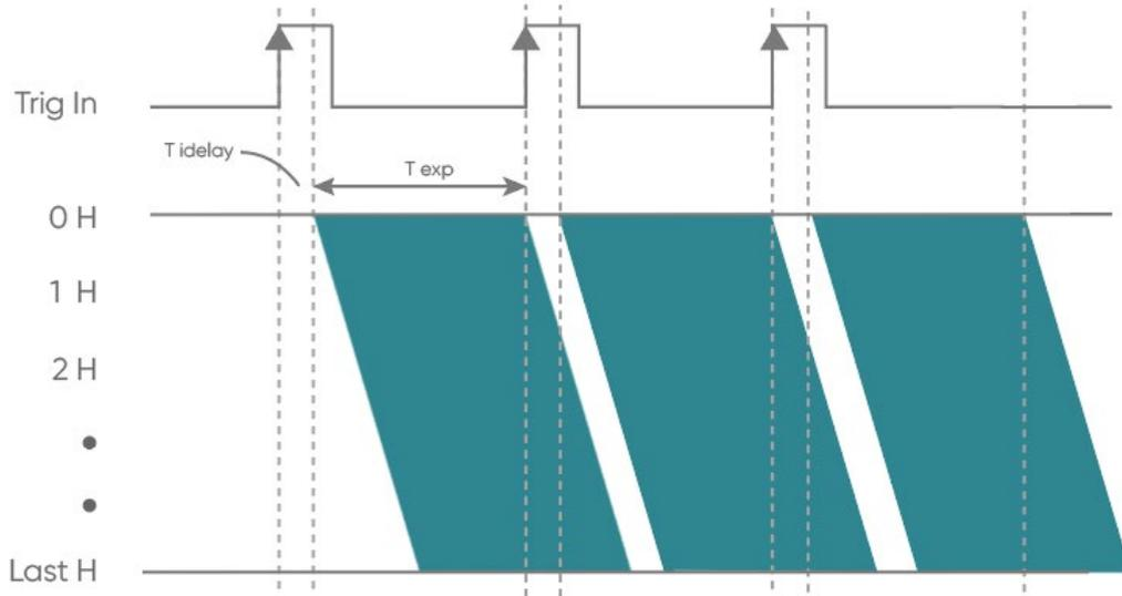
Figure 3-21 Standard (Overlap) Trigger timing
