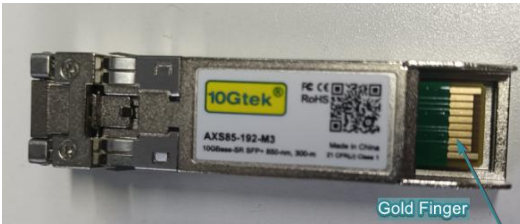
Figure 3-7 Direction of the gold finger of the optical module
