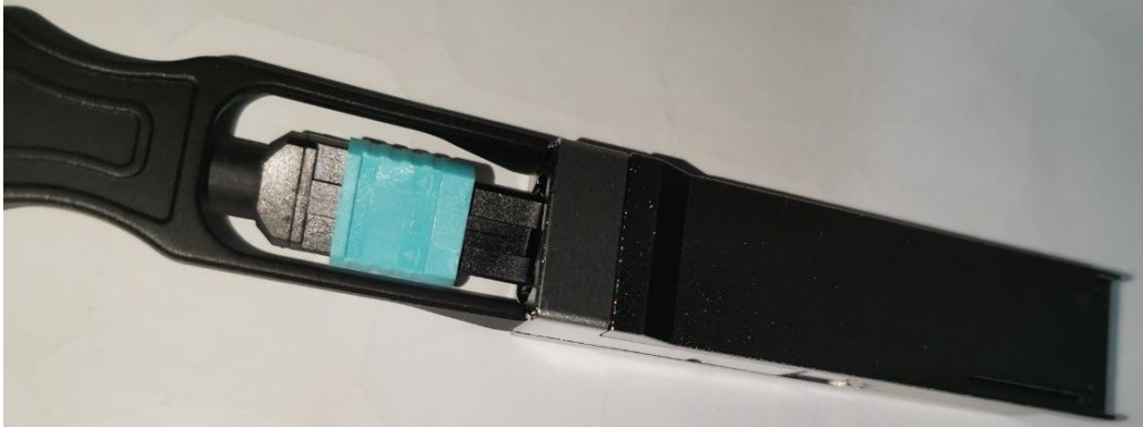
Figure 3-6 Connect optical fiber to QSFP+ optical module
