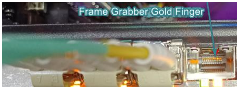
Figure 3-10 Direction of the gold finger of frame grabber
