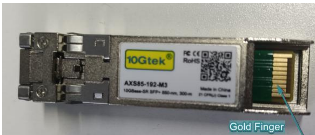
Figure 3-11 Direction of the gold finger of the optical module
