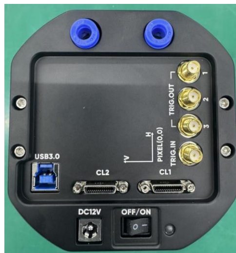
Figure 4-1 Schematic Diagram of the XF95 Camera Data Interface
