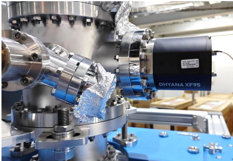
Figure 2-2 Schematic diagram of the camera outside the vacuum chamber
