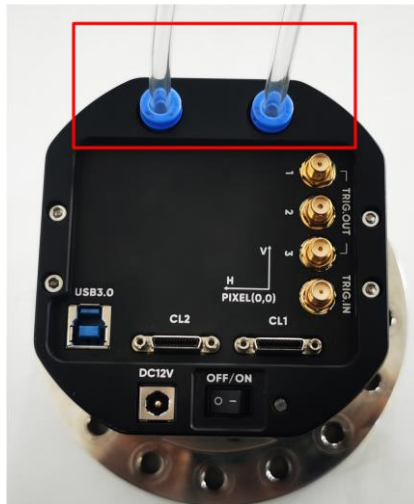
Figure 4-6 Camera end water pipe connector
