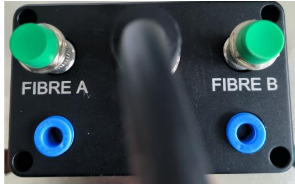
Figure 4-9 Atmospheric Side Flange Interface
