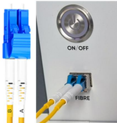
Figure 4-7 Connecting the LC fiber optic connector
