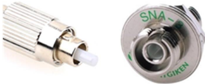
Figure 4-10 Connecting the FC connector
