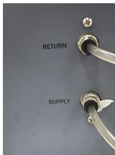
Figure 4-27 Cooling water circulator end water pipe connector
