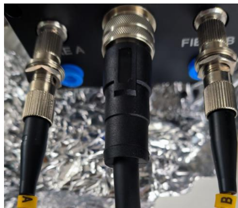
Figure 4-11 Atmospheric side of flange with connected cables
