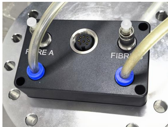
Figure 4-26 Camera end water pipe connector
