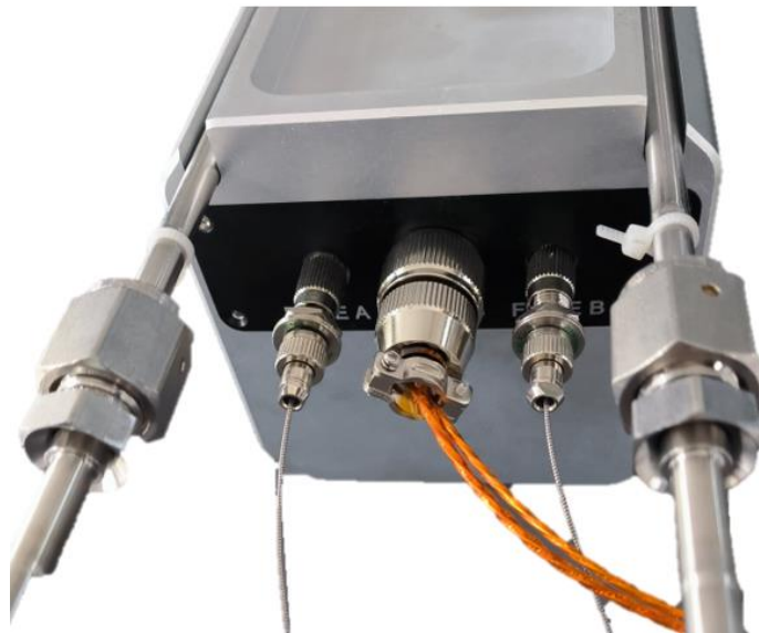
Figure 4-15 The camera with cables, optical fibers, and water cooling pipes connected
