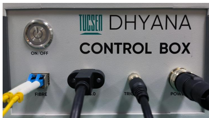
Figure 4-8 Control box with all cables connected
