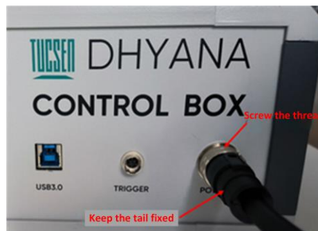
Figure 4-6 Power trigger cable connection
