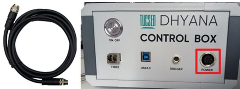
Figure 4-5 The vacuum cable (left) and the front (right) of the control box ( Outlined in red is the power socket)
