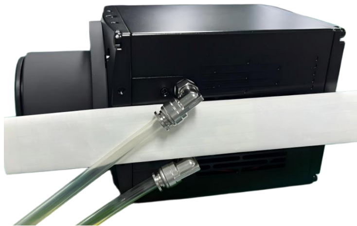
Figure 4-4 Removing water-cooled pipes
