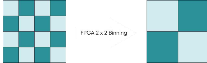
Figure 3-14 Schematic diagram of Binning
